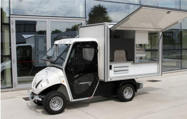
Padua, 5<sup>th</sup> September 2014 – The Alke' electric van with equipment for pizza is a real movable pizzeria. On the cargo bed are installed an oven (gas or electric), a double bowl sink with hot or cold water, a refrigerator, a work table, refrigerated containers for ingredients, a table for cutting and serving pizza.
